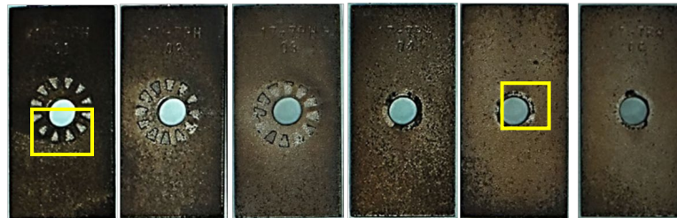
17Cr – 7PH After exposure (before cleaning)
