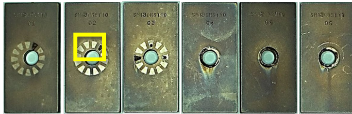
13Cr CRS 110 After exposure (before cleaning)
